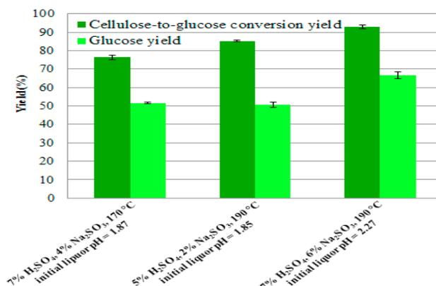
Fig. 2. Cellulose-to-glucose conversion and overall glucose yield through 48 h enzymatic hydrolysis of SPORL pretreated oil palm trunk under different pretreatment conditions
