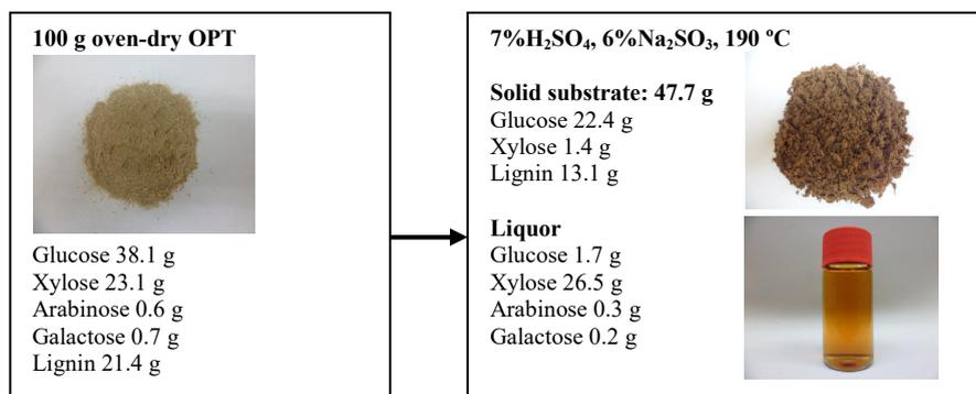
Fig. 1. Mass balance of SPORL pretreatment of OPT with 7%  $H_2SO_4$  and 6%  $Na_2SO_3$  at 190 °C for 30 min
