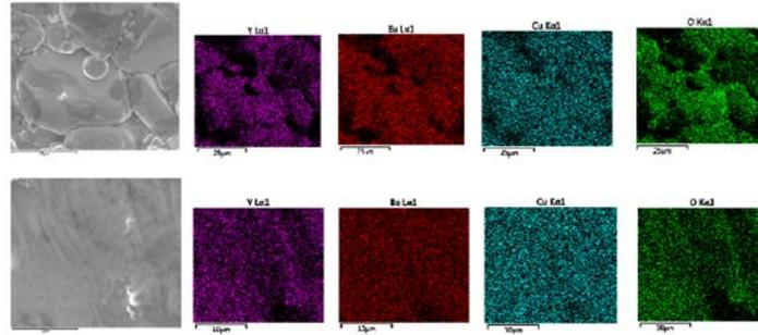
Figure 5. EDX mapping images of the melt Y5-8-13.
