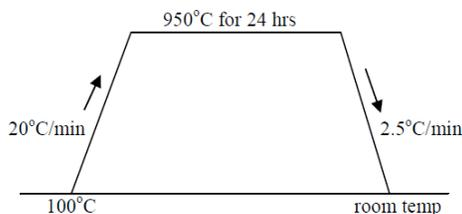
**Figure 1.** Schematic of the calcinations
