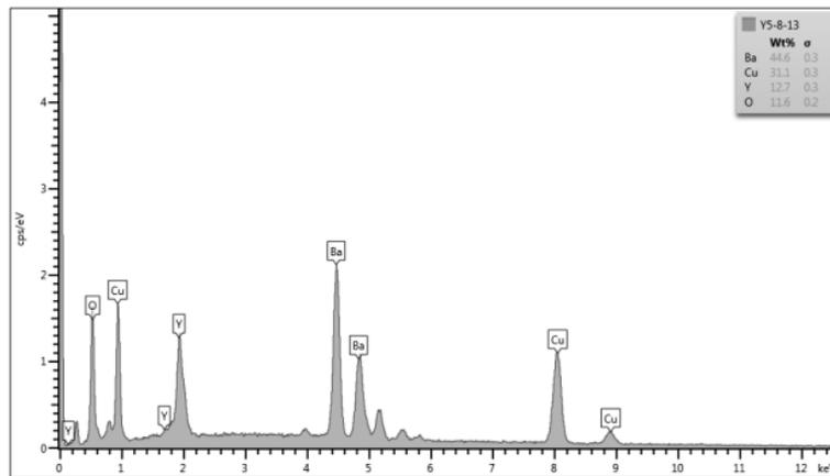
Figure 6. The EDX spectra of the melt Y5-8-13
