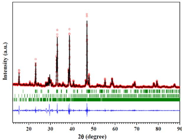
**Figure 4.** XRD pattern of melt Y5-8-13 superconductors.
