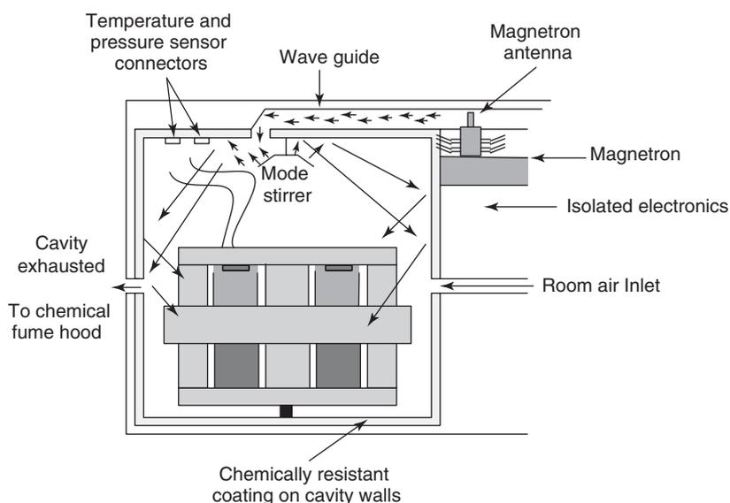
**Figure 2** Schematic diagram of a pressurized microwave-assisted extraction system.
