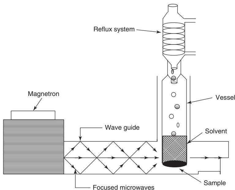
**Figure 1** Schematic diagram of an atmospheric microwave-assisted extraction system.
