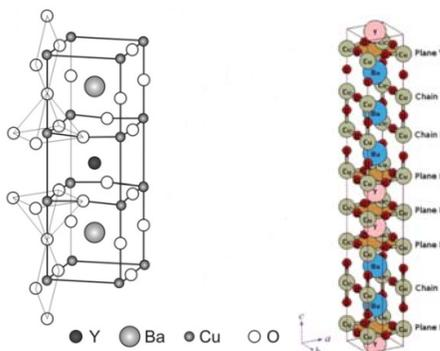
**Figure 1.** Crystal structures of  $\text{YBa}_2\text{Cu}_3\text{O}_7$  and  $\text{Y}_3\text{Ba}_5\text{Cu}_8\text{O}_{18}$
